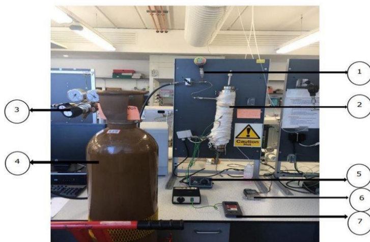
Figure 2. Experimental setup showing the gas permeation apparatus, including the pressure gauge (1), membrane module wrapped with heating tape (2), gas regulator (3), gas cylinder (4), temperature controller (5), volumetric flow meter (6), and temperature indicator (7).
