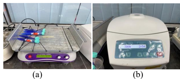
Figure 2 Diagram of adsorption experiment; (a) solutions were shaken by using an orbital shaker and (b) solutions were centrifuged after adsorption.
