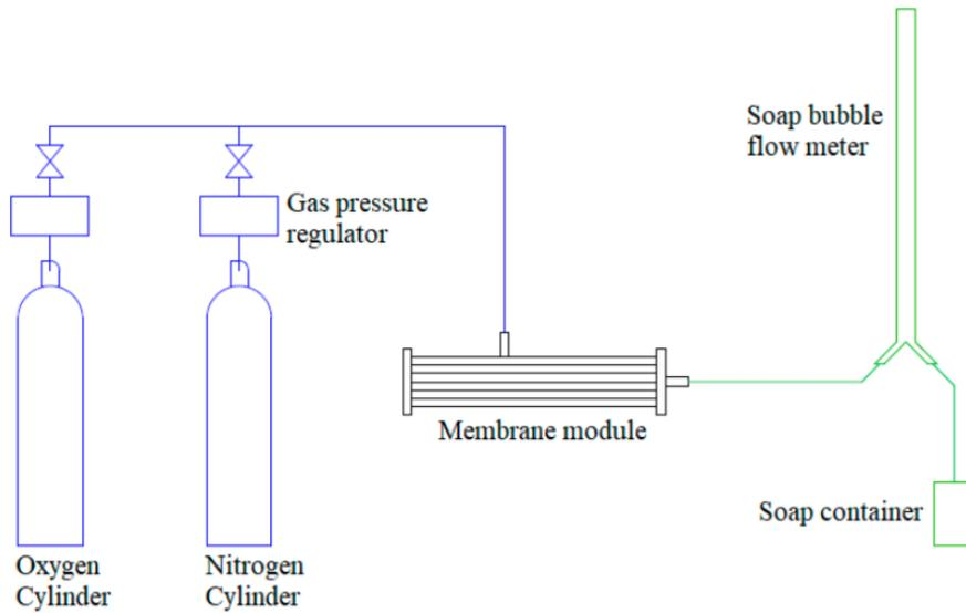
**Figure 2** The Schematic Diagram of Gas Permeation Study [15]
