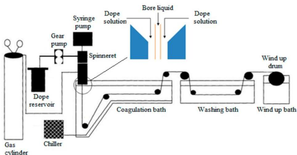
Figure 1 Dry-Jet Wet Phase Inversion Schematic Diagram [15]
