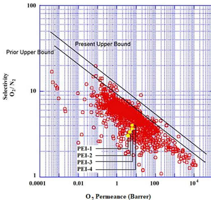
**Figure 4** Comparison of  $O_2/N_2$  gas separation performance in Robeson upper bound
