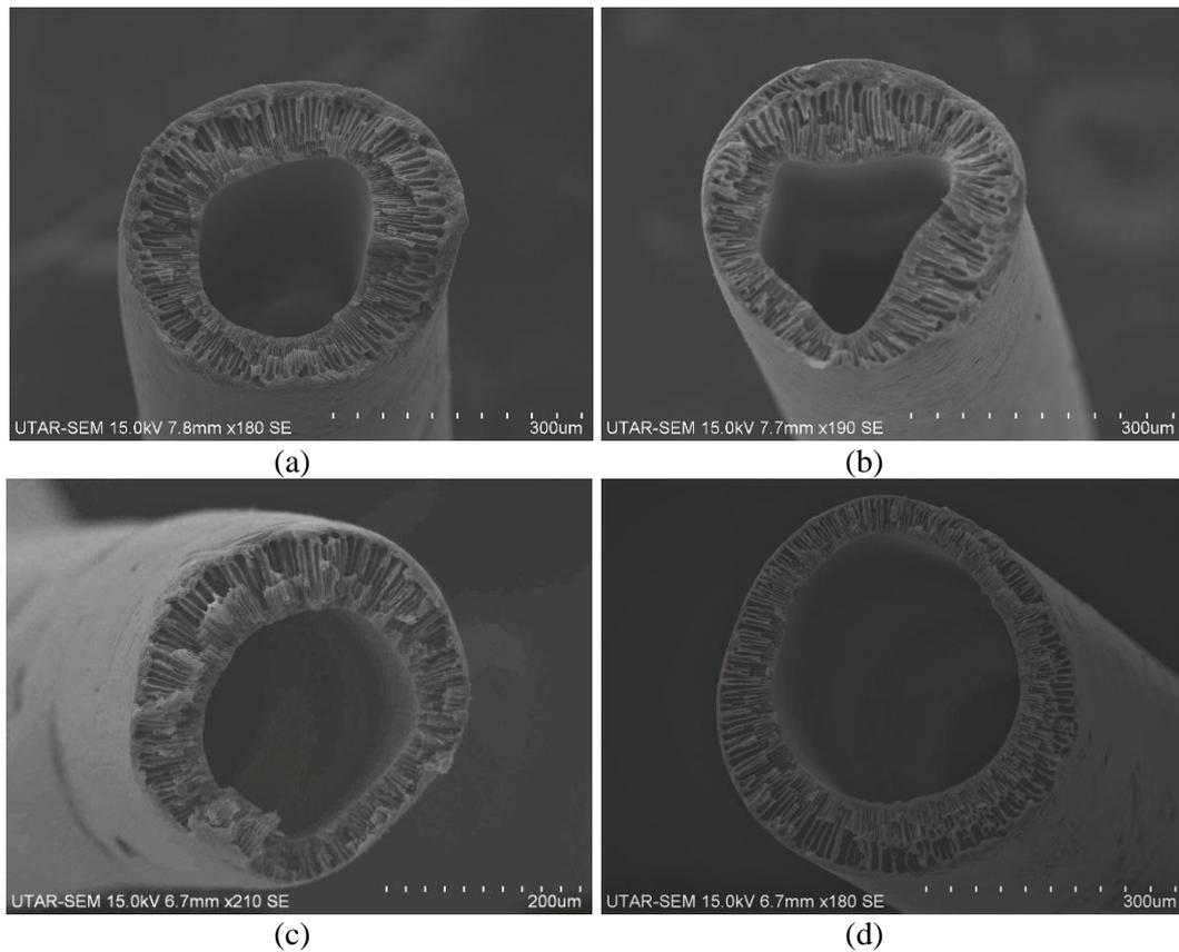
**Figure 3** SEM image of cross-sectional pristine PEI membrane under different spinning parameter (a) PEI-1; (b) PEI-2; (c) PEI-3; (d) PEI-4
